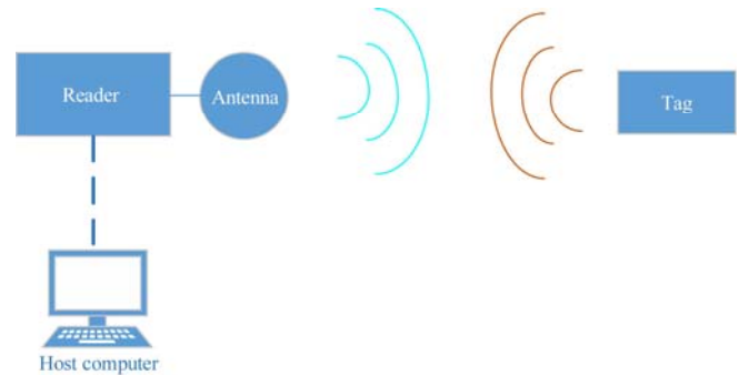
Figure 1 Architecture of a RFID system
