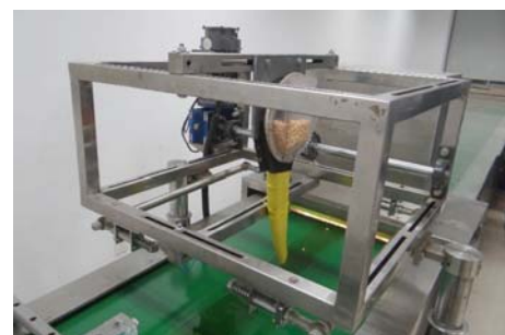
Figure 2 Type JPS-12 computer vision performance seed meter test bench
