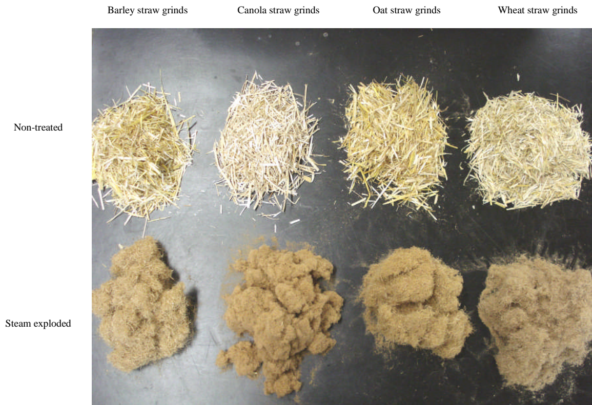
Figure 1 Non-treated (30 mm hammer mill screen size) and steam exploded barley, canola, oat and wheat straw grinds
