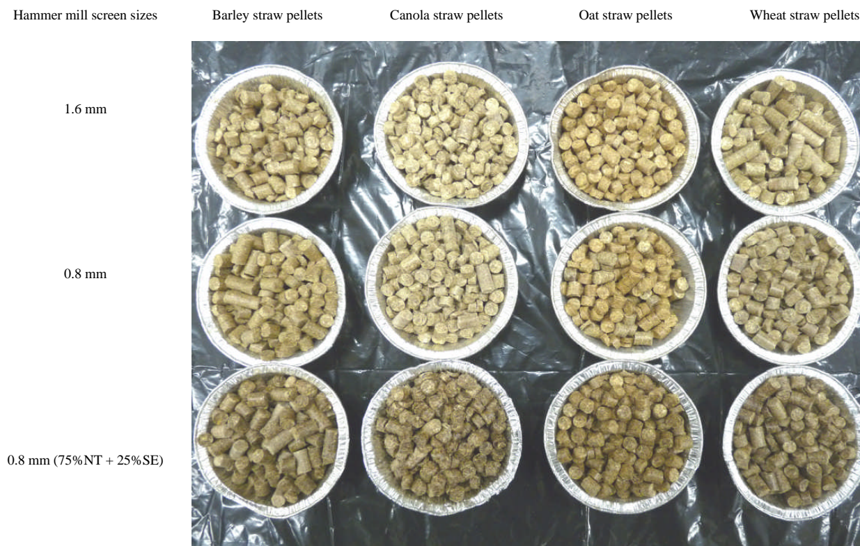
Figure 2 Photograph of pellets manufactured using a pilot scale pellet mill for non-treated (NT) straw at 1.6 and 0.8 mm hammer mill screen size, and customized grinds at 0.8 mm screen size having 25% steam exploded (SE) straw
