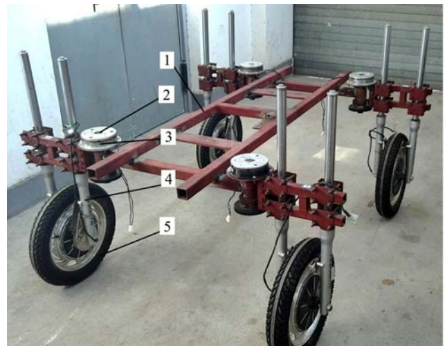
1. Chassis 2. Off-centered steering axis 3. EL 4. Shock absorber 5. IWM
