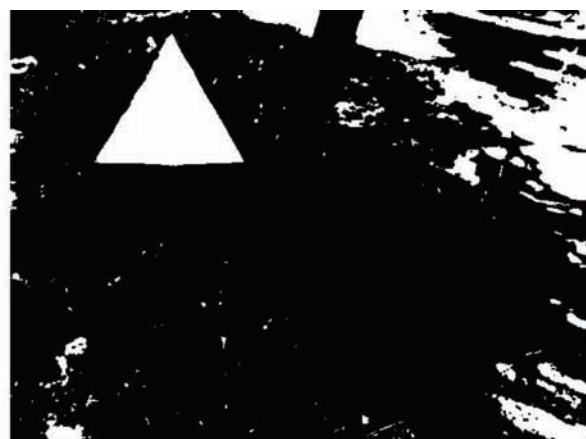
b. Binary result of threshold which needs further process including dilation and erosion to filter small object
