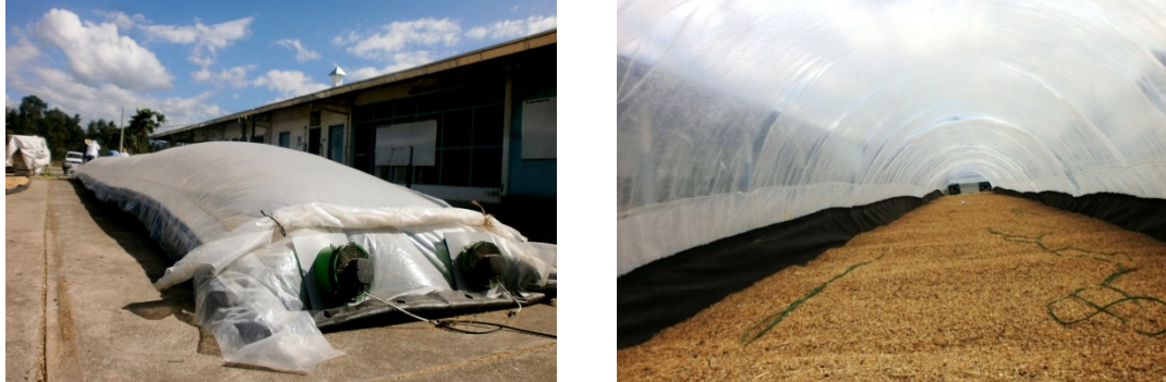
Figure 1 Images showing external (left) and internal (right) views of the inflatable solar dryer
