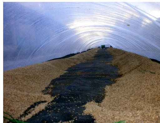
Figure 11 Condensation along the drying area ISD during the rainy season experiments (paddy is moved aside to show the wet areas)
