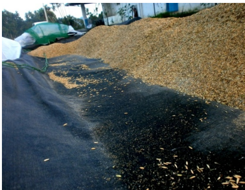
Figure 11 Condensation along the drying area ISD during the rainy season experiments (paddy is moved aside to show the wet areas)
