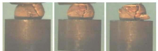
a. Start b. Shell breaking c. Shell and kernel separation
