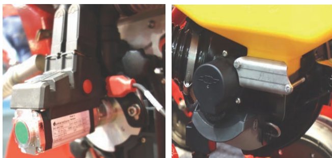
Figure 3 Seed meter driven by motor with gear reducer on shaft
