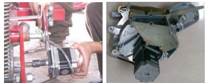
Figure 5 Seed meter driven by high-torque motor on shaft without gear reducer
