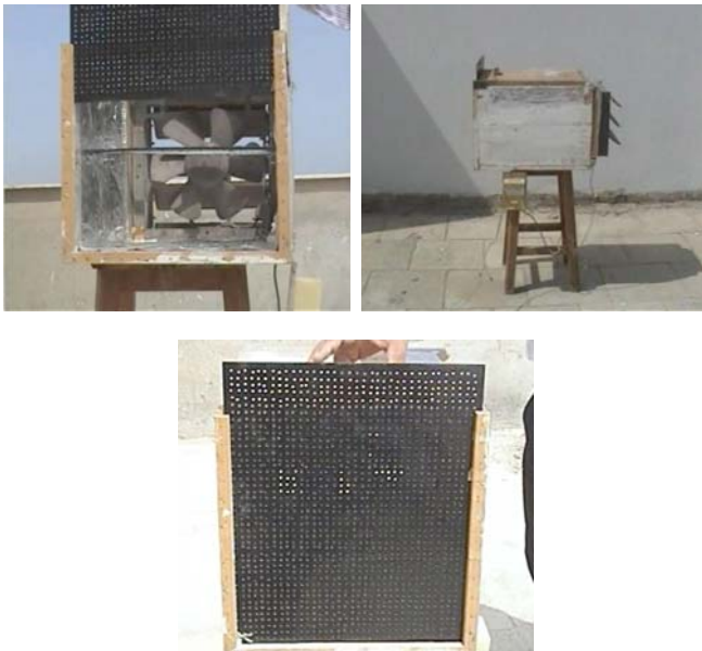
Figure 2 Rig-setup for the field investigation
