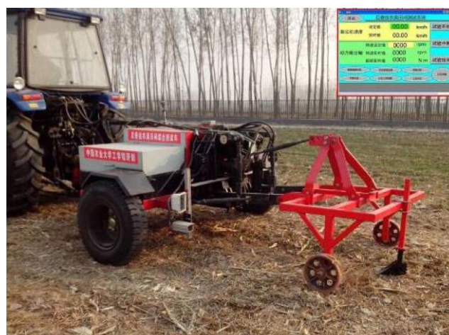
Figure 3 Furrow openers tested by field integrated testing system
