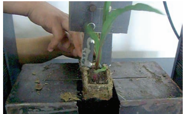
Figure 11 Performing the cutting seedling-growing tray experiments
