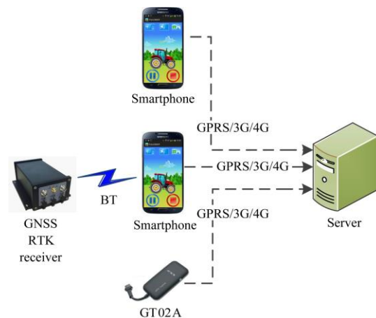
Figure 5 Wireless data transmission
