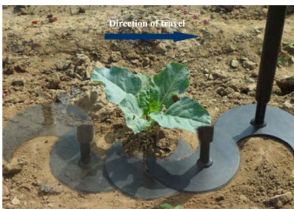
Figure 2 Weeding blade rotates to avoid hurting crop plant
