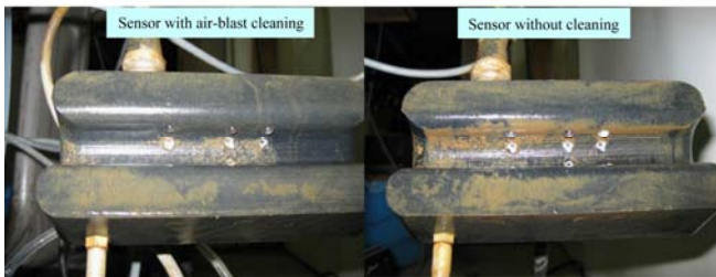
Figure 11 Polyethylene sensors after working in water for 18 d
