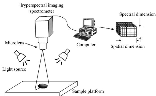
Figure 1 Hyperspectral imaging system
