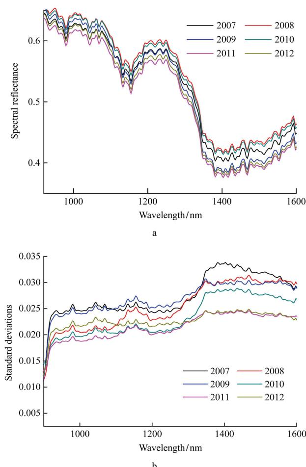
Figure 4 (a) Spectral reflectance of the grains stored for different years; (b) Standard deviations of spectral reflectance of the grains stored for different years
