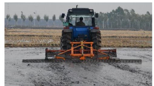
Figure 1 Structure diagram and working condition of 1JPS-600 puddling and flatting machine for paddy field
