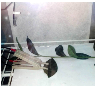
Figure 2 Leaf clamping by the test probe
