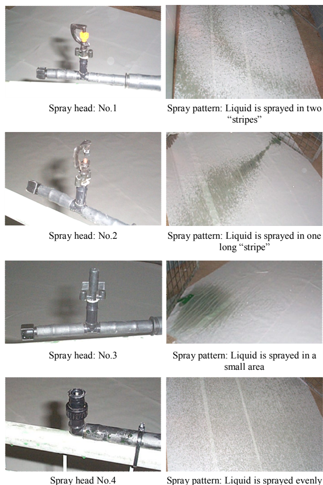
Figure 1 Different spray heads used during this study and the respective spray patterns
